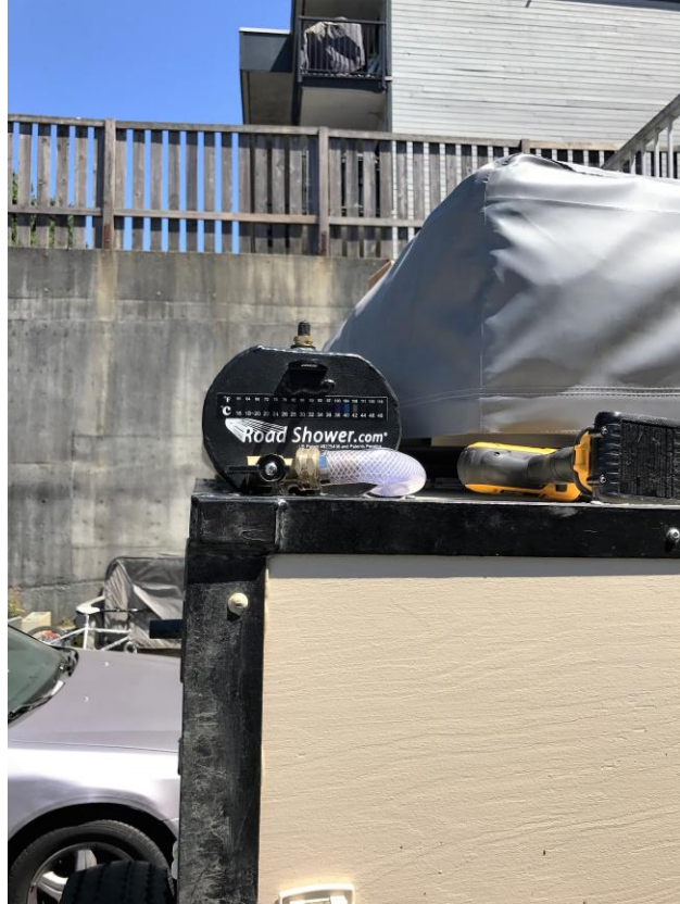
18 - Grabbed a solar water heater from one of the Overlanding shows we attended this year. Works pretty good! Still trying to figure out how to keep it pressurized. It would appear the "rad cap" supplied with the shower, only supports up to a maximum of 25psi..... I'm going to try and find one that's at least double!
