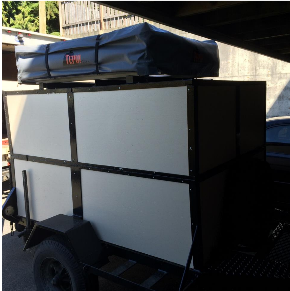
16 - The final assembly of the walls - complete
